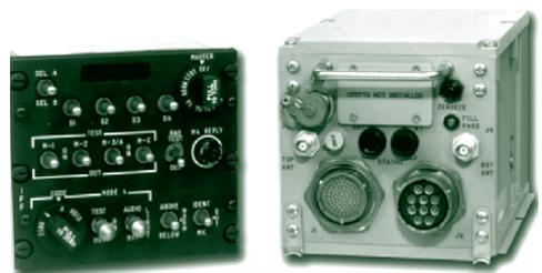
Figura 8: Interface homem-máquina do IFF AN/APX-100 Mark XII/Mode S IFF *Transponder*.
